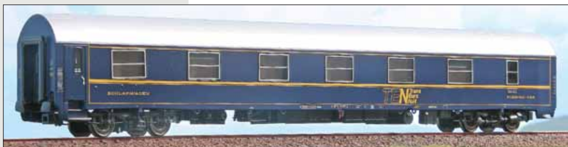
Carrozza letti MU Tipo 1973 nella livrea intermedia (CIWL-Pool) applicata su alcune unità del parco SNCF. Type MU 1973 sleeping car wearing CIWL-Pool livery used on few units of the French fleet. Schlafwagen type MU 1973 der SNCF mit ISG-Pool sonder Lackierung.
